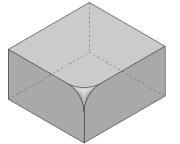
7. Enter *Radius* 10, collect edge 1, 2 and 3. Release on required position by clicking the mask on edge 1 and 2, enter *Radius* 0, release any on edge 3.
