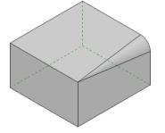
9. Identify edge 2. Enter *Radius* 15, enter *Position* 0, enter *Radius* 5, enter *Position* 0.3, enter *Radius* 10, enter *Position* 0.7, enter *Radius* 0, enter *Position* 1,
