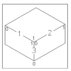
Origin solid with edges 1, 2, 3 and the positions 0 or 1 on the endpoints of each edge.
