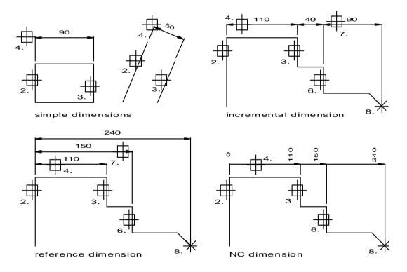
The dimensions listed here will be computed orthogonally in each case, i.e. horizontally or vertically. They can be defined as a simple dimension, incremental or a reference dimension:
