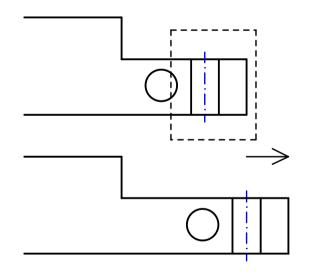
If there is only one endpoint of each line inside a window, this point will be moved, whilst the other will stay where it is.
