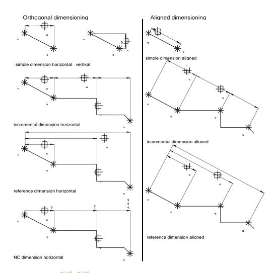
1. 🕅, 🕅 Use the command *Dimension, Orthogonal Multi Dimension* to dimension the horizontal or vertical distance of points and if applicable extend it to a string or reference dimension.
