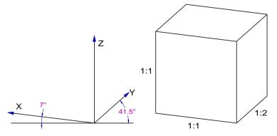
The predefined dimetric views rotate the view of the model in the direction of the angle relative to the global 3D coordinate system with the angle aligned to the right or left.
