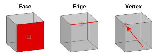
The options on this option card can be used to **blend** two faces, two edges or a face and an edge.
