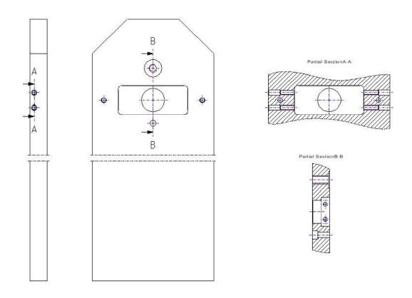
In order to be able to create partial cuts of objects, a model view must have previously been inserted into the 2D drawing window using the menu command *Insert*, *Model Views*.
