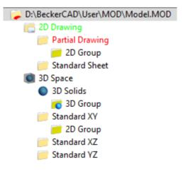
The 3D space contains the necessary **workplanes** (WP) for the generation of 2D objects and solids. After starting the WPs *Standard\_XY, Standard\_YZ* and *Standard\_XZ* are available. Whilst the 2D objects in 3D space are linked to the WP on which they have been generated, the solids and the 3D polygons are managed completely independently in the **3DGroupStructure** section that can also contain groups for these 3D objects.
