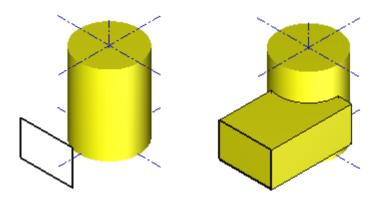
*Height 1* will, in this case, determine the extension of the swept solid, if it runs, in part at least, close to the target solid.
