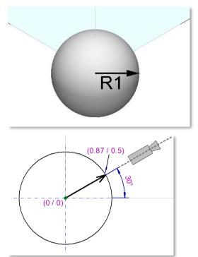
The coordinates in the *Presentation mode* dialog for the viewing direction show the end point of a vector with length 1 whose starting point is at the absolute zero point. This vector determines the viewing direction. A viewing direction, starting from the view from the left, rotated by 30° to the right, results, for example, in the coordinates (0.87,0.5,0).
