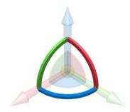
If this setting is activated, you can only rotate the 3D gadget after clicking on an arc at angles that are multiples of the entered value. This setting is ignored if the point definition menu is used to capture a point on an existing object, the status window is used to define a different angle, or the *Shift* key is held down.
