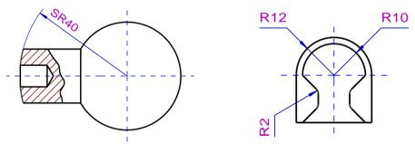
N. N. K. Activate the command by clicking the icons *Dimension, Multidimension Orthogonal* or the icons *Dimension, Multidimension Aligned* or call up the command *Dimension, NC Dimension*.
