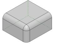
4. Enter *Radius* 10, collect edge 1 and 2, *Accept*. Deactivate *sequential*, identify edge 3, *Accept*.
