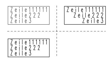
With the options for the mirror behavior of texts "modify position" and "modify position and reference point" the text was aligned in the way that it could be read "from below".
