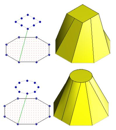
With this type of connection a point on the perimeter of one of the faces will be paired with a point on the perimeter of the other face. The program starts from this connection to determine the positions of the remaining compulsory points and connects them with solid edges.
