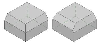
Collect edges 1, 2 and 3, enter Left dist. 10, Right dist. 15, release on edges 1 and 2 by clicking the mouse. Enter Left dist. 10, Right dist. 10, release on edge 3 by clicking the mouse, Accept.
