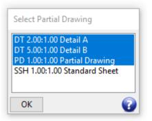
Tag all the partial drawings that are to be taken into consideration during the selection procedure by clicking them with the cursor. You can remove the tag from a partial drawing by clicking a second time.
