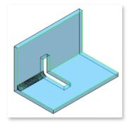
6. The blending is bordered where one of the contact tracks meets a sharp edge.
