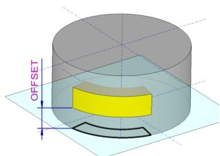
4. If the swept solid should be created with a distance to the active plane, please define an *Offset* in the status dialogue window, for the distance between the base face of the swept solid and the 2D face or the planar surface.
