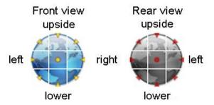
These icons can be used to select the main view directions named in the illustration and also to select the combined view directions such as from front, left and top.
