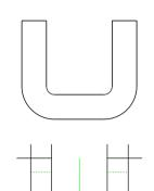
4. If the face for the solid is not yet defined as a 2D face select the 2D contour elements by collecting with the pressed *CTRL* key or by dragging a window. The selected elements should clearly define a closed contour. Overhangs, branches and intersections to other objects should be avoided.
