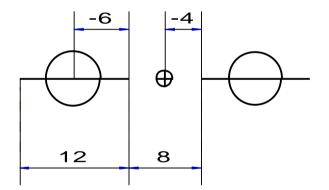
If a value of > 0 is entered for the width, the partial elements, which have this width, are displayed. If the value 0 is entered, they are displayed with a width, which is set in relation to the layers or objects.
