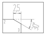
If a *chamfer length* and *chamfer angle* have been predefined on the *2D draw* option card using the menu command *Settings*, *3D/2D Commands*, these values are displayed in the Status dialog box.
