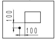
In this case, a drawing with the dimensions of an A4 sheet (297 x 210) is moved starting from the origin by 100 units in the direction of both the X and Y axes. This means that the left bottom corner of the drawing now has the coordinates (100, 100) in the GCS, the top right corner has the coordinates (397, 310).
