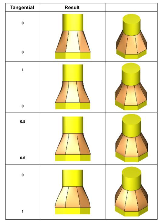
**9.** Activate the appropriate option in the tab <u>Parameter</u>, to get the desired result.
