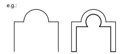
6. You can use the cursor to specify the position of the parallel continuous line dynamically or you can enter a value denoting the *Distance 1* in the Status dialog box.
