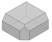
**5.** Collect edge 1, 2 and 3, *enter Left dist.* 10, *Right dist.* 15, release on edges 1 and 2 by clicking the mouse.
