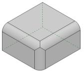
5. Enter *Radius* 10, collect edge 1, 2 and 3, on edges (1, 2, 3) for the common corners in the text boxes (*Indent 1*, *Indent 0*, *Indent 0*) enter the value 15.0, *Accept*.
