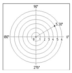
When using polar coordinates, each point in the plane is defined by a distance and an angle from the origin of the selected coordinate system. The angle is taken from an angle of 0° to the "right" or "east" of the origin in an anticlockwise direction.
