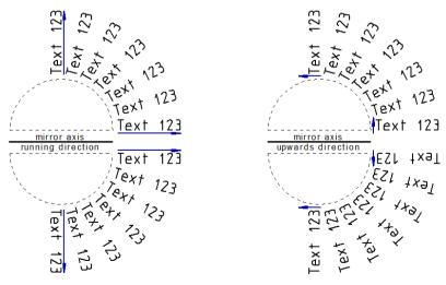
u d In the parameter dialog box *Referenced Texts / Position Numbers* the display of referenced texts and position numbers can be saved in different display styles.
