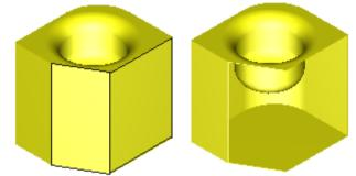
Identify the faces to be removed or identify the faces which are to be retained and reverse the selection by pressing the  $\underbrace{\mathbb{N}}$  icon of the context dialog box.
