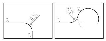
If a *blend radius* has been predefined on the *2D draw* option card using the menu command *Settings, 3D/2D Commands*, this value is displayed in the *Radius* text box in the Status dialog box.
