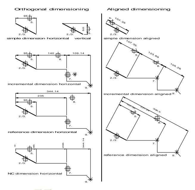
1. Activate the command *Dimension, Multidimension Orthogonal*, if the horizontal or vertical spacing between the endpoints of a line are to be dimensioned and, possibly, to be expanded to a reference dimension or an incremental dimension. Activate the command *Dimension, NC Dimension*, if the horizontal or vertical spacing of the endpoints of a line are to be dimensioned and, possibly, be extended to an NC dimension.
