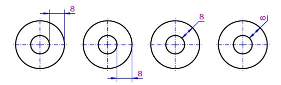
6. Define the position of the dimension line by cursor or by entering a value in the filed *distance* of the status dialog window.
