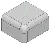
6. Enter *Radius* 0, collect edge 1, 2 and 3, position cursor on each edge and release the radius at any position with a mouse click. On edges (1, 2, 3) for the common corners in the text boxes
