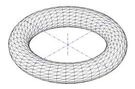
Here you can set the precision with which shaded solids are to be presented with curved surfaces. It does not affect the accuracy of which the geometric data of the solids are managed.
